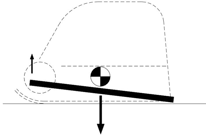
In the case of reversible plates, excitors are usually located very near the center of gravity and amplitude tends to be equal over the surface of the plate.. The same amplitude formula for vibratory plates applies to reversible plates, but in this case the result can be described as maximum amplitude. See figure below:
