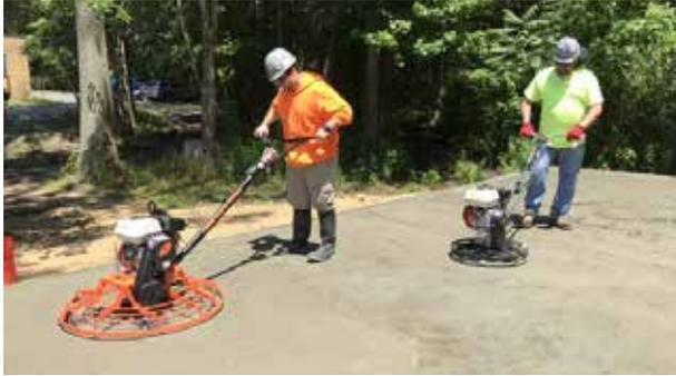
The F24 EDGER TROWEL is ideal for jobs that require a lightweight, highly maneuverable, professional finishing tool. This specialty finishing power trowel allows professional results even when confined areas or weight restrictions leave other machines standing idle. Perfect for edging in the tightest spaces, the F24 Walk Behind Power Trowel is always ready when needed.
