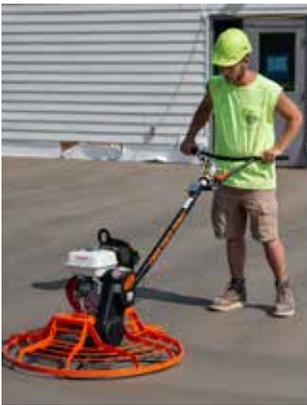
To function properly, power trowels must maintain a precise perpendicular relationship between the gearbox's output shaft and blade arms. Once that relationship is compromised, the trowel will vibrate and/or wobble. MBW has gone to great lengths to maintain this critical relationship.
