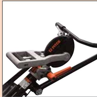
*The EZ Pitch™ handle employs a constant force gas spring to allow for low effort and rapid adjustment of blade pitch. Can be retrofitted to older MBW trowels as a complete assembly.*
