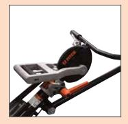
The EZ Pitch™ handle employs a constant force gas spring to allow for low effort and rapid adjustment of blade pitch. Can be retrofitted to older MBW trowels as a complete assemby.
