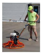
To function properly, power trowels must maintain precise perpendicular relationship between gearbox's output shaft and blade arms. Once that relationship is compromised, the trowel will vibrate and/or wobble. MBW has gone to great lengths to maintain this critical relationship.
