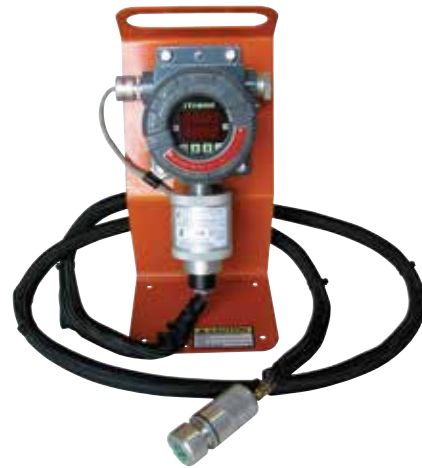
LEL SENSOR PROVIDES REAL TIME DIGITAL READOUT OF GAS CONCENTRATION AND INITIATES ALARM AND/OR AUTO SHUT DOWN SHOULD GAS LEVEL EXCEED SELECTED THRESHOLDS. OPERATOR ADJUSTS GAS/AIR MIXING VALVE TO MAINTAIN GAS CONCENTRATION WELL BELOW LEL.
