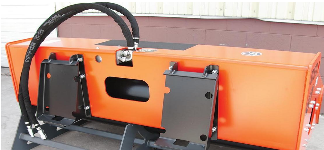
Previous design with mating portion of the hitch attached to the frame
